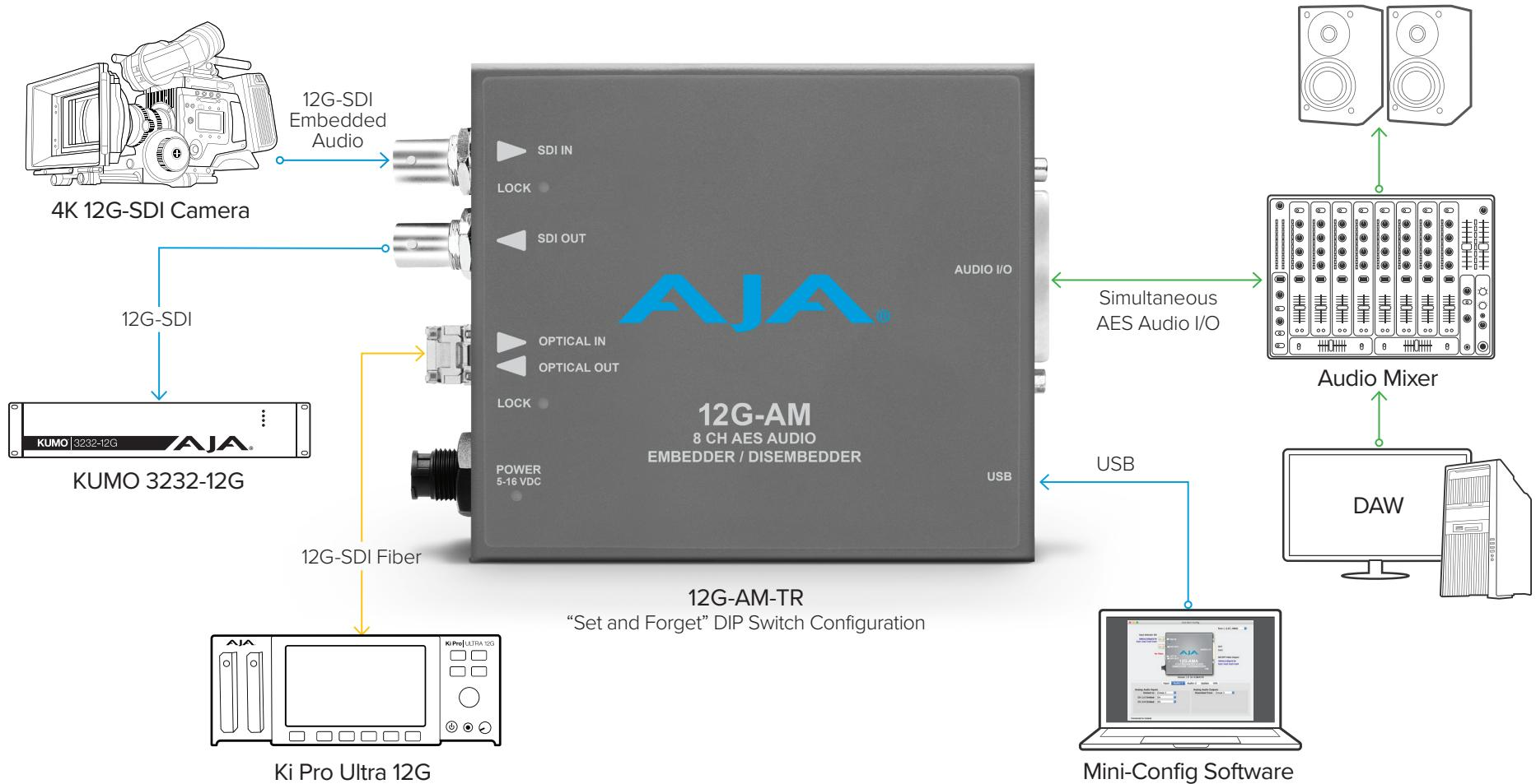
Simultaneous Embed/Disembed to/from 12G-SDI with Optical Fiber I/O
